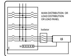
4.4.2 **Surge source installation:** Install Surge Diverter at load distribution or load panel to protect surge from the START-STOP equipment or in the special protection areas such as signal control room and server room.
