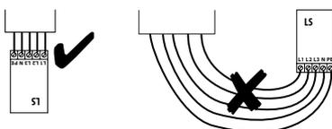
4.3 In case that it is not possible to wire the system with 25 cm. cable length, use 2 sets of 4 mm<sup>2</sup> cables which each length is shorter than 50 cm. Split them into 2 sets (L1,L2,L3, N and G/PE) with minimum space 10 cm. or 4 inches. Tie the cables with cable tie or spiral wrap for the whole length.
