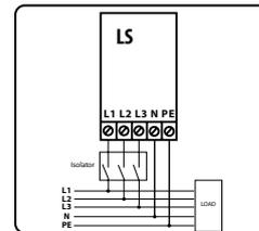
4.5 Recommend to install a circuit breaker to separate Surge Diverter from electricity system for maintenance and protection of the cables from the surge diverter to the electricity system.
