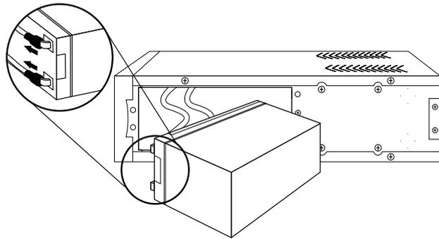
5.5.3 Replace new battery by reconnect the black (-) and red (+) wire to the battery terminals respectively.
