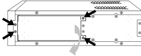
5.5.2 Tilt the UPS and gently pull the battery out of the UPS. Then, disconnect black and red wires from the battery terminal respectively.
