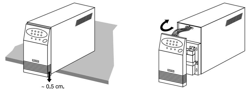
9.3 Stand the UPS up, unscrew the screw on the battery strip.
