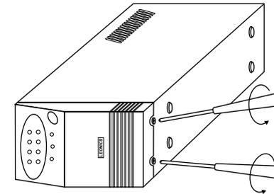
9.2 Stand the UPS up, place it at the edge of a table. Bulge its front panel from the edges and slide the front panel up about 0.5 centimeter and pull out as shown.
