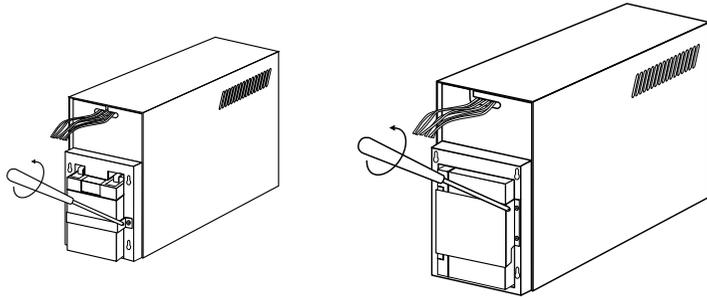
9.4 Remove the battery terminal cover. Disconnect the black and red wires from the battery terminals. Then pull the battery out and replace with the new one. For the 1050VA or higher model, please notice each connection carefully before replace the new one.
