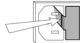
10.4 Check the fuse in whether it is blown. Replace the blown fuse with the spare fuse.
