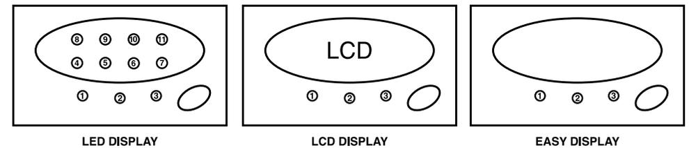
3.1.1 **Multi-function Switch:** The switch to turn on, turn off, test the UPS and mute the audible alarm. For LED Display UPS, you can press it to change the display mode from input voltage - load level mode to battery voltage level mode and vice versa.
