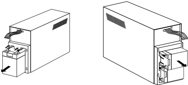
9.5 Reconnect the black and red wires to the black and red terminals. For 1050VA or higher model, reconnect each wires connection to each battery same as before.
