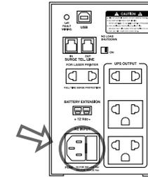
10.3 Use a flat head screwdriver to release fuse holder from its compartment.
