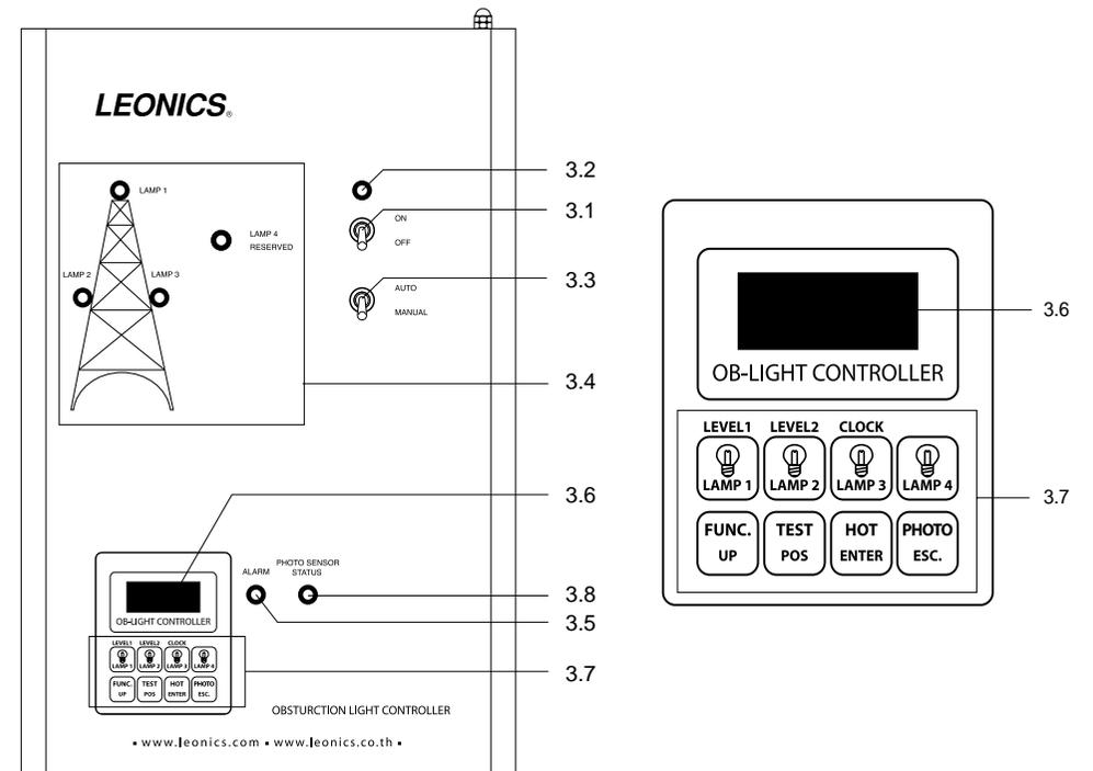
**3.1 ON/OFF Switch :** The switch to turn on and off OBSTRUCTION LIGHT CONTROLLER.
