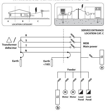
4.4.2 <u>Surge source installation</u>: Install Surge Diverter at load distribution or load panel to protect surge from the start-stop equipment or in the special protection areas such as signal control room and server room.
