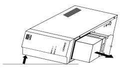
6.3 Disconnect the black and red wires from the battery terminals respectively. Then pull out the battery and replace the new one.
