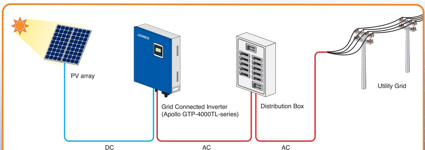
The APOLLO GTP-4000TL series inverter is high performance three phase grid connected inverter that integrated with PV maximum power point tracking (MPPT) to extract maximum DC power generated by PV array. It can operate at their optimum power output voltage even under variety weather conditions and also offers user-friendly and high efficiency circuit design. With real-time monitoring software, the inverter can help users to monitor and calculate the accurate saving energy.
