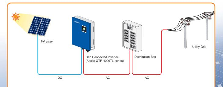
The APOLLO GTP-4000TL series inverter is high performance three phase grid connected inverter that integrated with PV maximum power point tracking (MPPT) to extract maximum DC power generated by PV array. It can operate at their optimum power output voltage even under variety weather conditions and also offers user-friendly and high efficiency circuit design. With real-time monitoring software, the inverter can help users to monitor and calculate the acurate saving energy.
