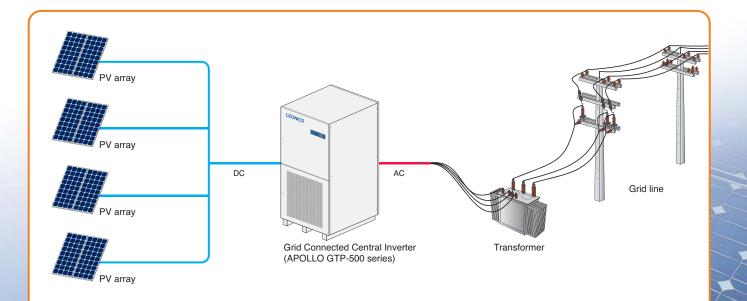
The APOLLO GTP-500 Series is high performance three phase grid connected central inverter that integrated with PV maximum power point trackers (MPPT) to extract maximum power generated from the PV arrays, and also system protection during failure of utility grid power supply. The APOLLO GTP-500 series inverter is suitable for medium to large scale grid connected solar power system.
