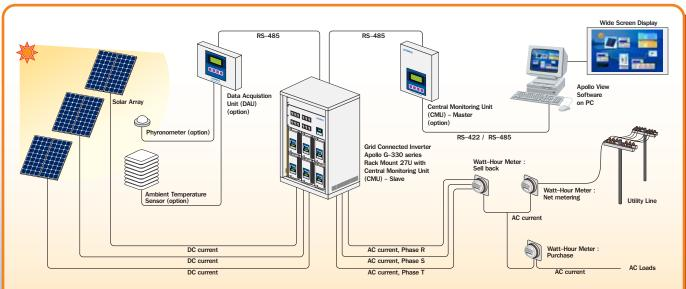
With a Grid Connected Solar Power System, clean solar power takes the place of grid power when the sun is shining, even to the point of selling a surplus back to grid. When the sun is not shining or when extra power is needed, electricity can be automatically purchased from the grid.
