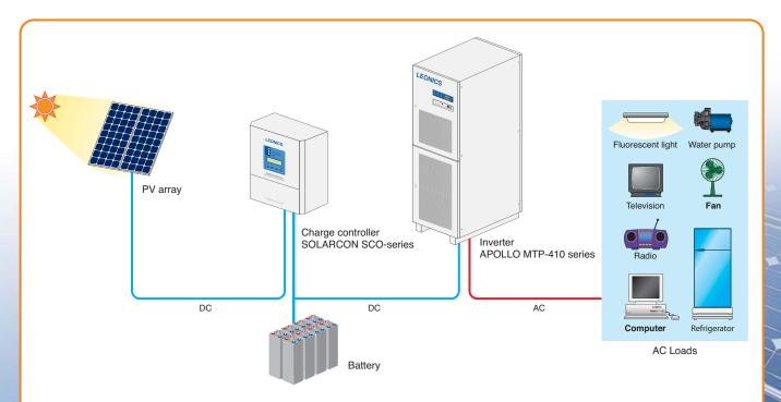
The SOLARCON SCO-series charge controller is the most sophisticate solar charger with PV Maximum Power Point Tracking (MPPT) algorithm. The charge controller equipped with advanced microprocessor control to get the maximum power from PV to charge battery with LCD display and front panel for easy and accurate setting more over the digital meter with 180 days power and event logger are inclusive.
